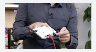
Use the EBS Power Supply to provide the Base Station with 6V power. You can use the EBS Ethernet cable to connect the Base Station to your existing network. A demo set of 5 NFC cards with Opticon Print are available. You can program these cards with the NFC Reader.
